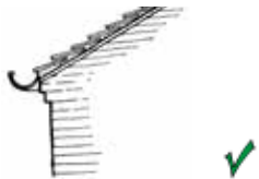
Clipped / parged eaves
