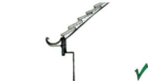
Shallow, black fascia / barge board on eaves
